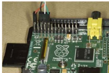
How to connect the serial-USB adaptor
